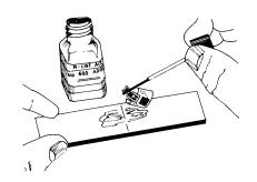
Now, by lifting at a shallow angle, peel back one end of the taped assembly so as to raise both gage and terminal. By curling this mylar tape back upon itself, it will remain in position, ready to be accurately repositioned after application of adhesive.
