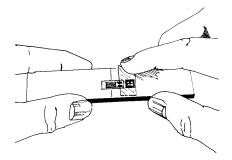
Remove the gage/tape/terminal assembly by peeling the tape at a shallow angle (about 30°) and transferring it onto the specimen. Make sure gage alignment marks coincide with specimen layout lines. If misalignment does occur, lift end of tape at shallow angle until assembly is free. Realign and replace. Use of a pair of tweezers often facilitates this handling.
